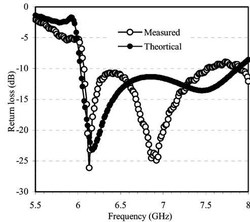
Fig. 3. Measured and theoretical return loss of the antenna.
