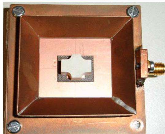
Fig. 1. (a) Cross DRA on patch with SMSH. (b) Photograph of a prototype.
