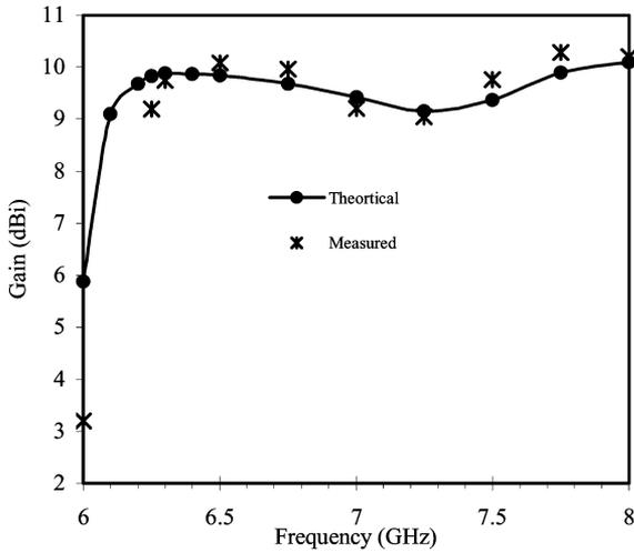
Fig. 4. Theoretical and measured gain of the antenna.
