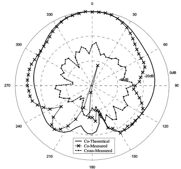
Fig. 6. (a) E-plane radiation pattern at 7.25 GHz. (b) H-plane radiation pattern at 7.25 GHz.
