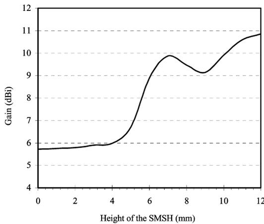
Fig. 2. (a) Gain variation with the height of the SMSH and frequency for  $b = 27$  mm,  $d = 32$  mm and  $\theta = 45^\circ$ . (b) Gain variation with the SMSH length. Width of the SMSH  $d = b + 5$  mm. (c) Theoretical gain of the antenna at 7 GHz.
