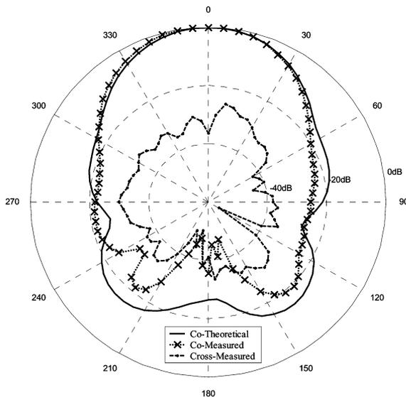
Fig. 5. (a) E-plane radiation pattern at 6.25 GHz. (b) H-plane radiation pattern at 6.25 GHz.
