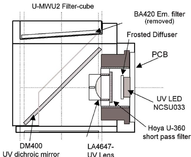
**Fig. 2** Cutaway view of the U-MWU2 Olympus filter cube illustrating the optical components of the Nichia NCSU033 UV LED excitation scheme. Due to the narrow passband of the LED emission, both the excitation and emission filters were removed from the filter assembly for this work.
