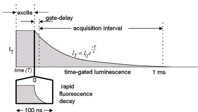
**Fig. 1** TGL suppresses autofluorescence by delaying signal acquisition until prompt (auto-fluorescence) has faded. Lanthanide chelate luminescence can persist for milliseconds, greatly facilitating its detection in the absence of autofluorescence.
