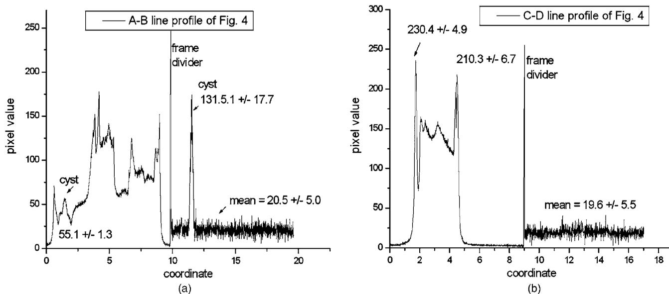
**Fig. 5** (a) Line profile A-B was sampled to compare pixel values on the labeled cyst for prompt and TGL modes. (b) Second line profile C-D in Fig. 4 transits a strongly fluorescent region that was used to determine the effectiveness of TGL suppression. Data from both regions was used to calculate the improvement in SNR (30-fold).
