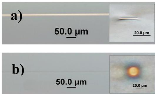
Figure 2: Differential interference contrast (DIC) microscope images of waveguides fabricated in phosphate glass using a) a standard spherical focusing geometry and b) the slit beam shaping technique.
