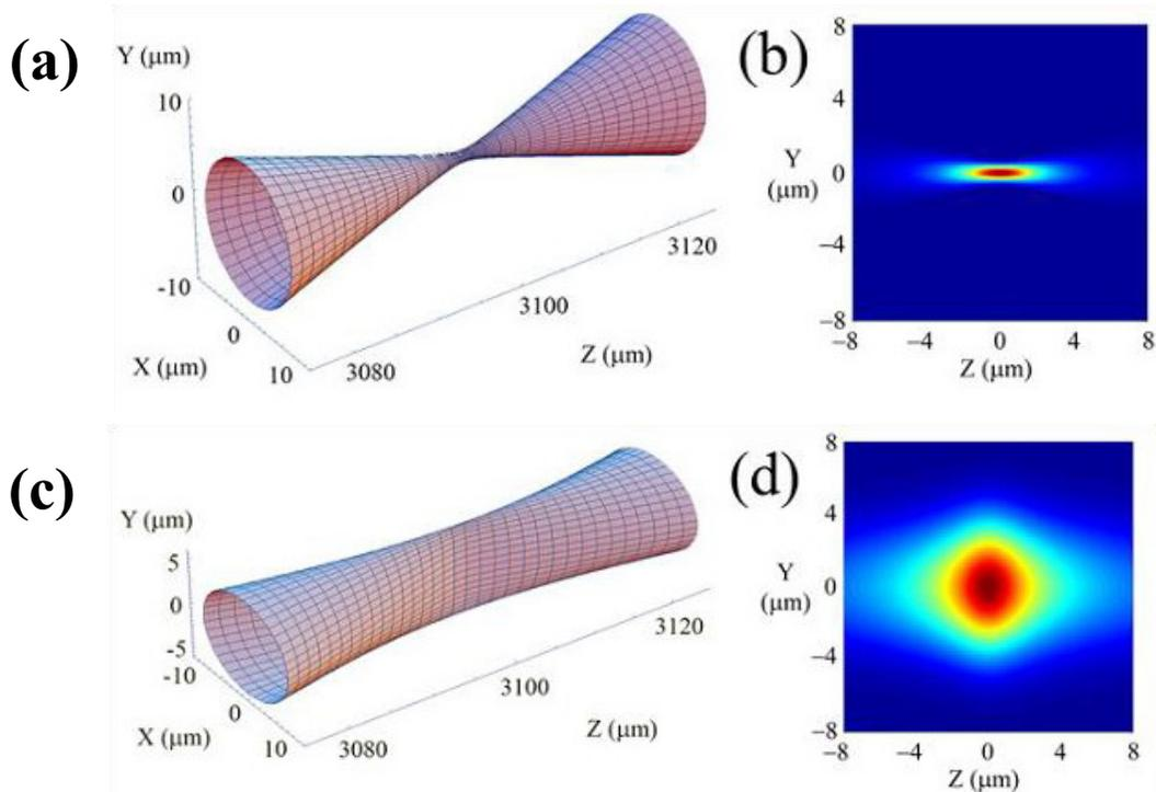
Figure 1: Beam evolution (a) and energy distribution in the YZ focal plane (b) when using a standard spherical focusing geometry. Beam evolution (c) and energy distribution in the YZ focal plane (d) when beam shaping using a slit.
